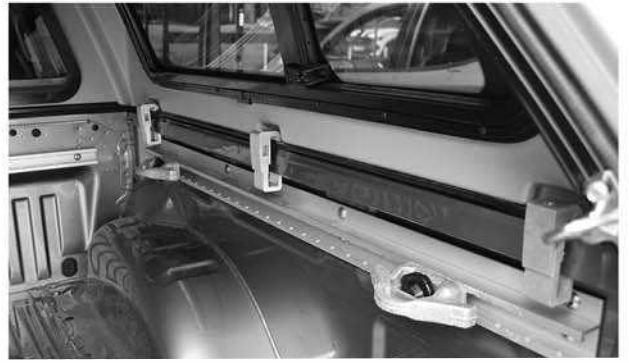
Image showing clamps fitting onto the canopy above the C-Channels and not into them.
